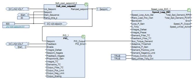
The *Soft Start Setpoint* FB allows the PID setpoint to be ramped from starting value (~480V in the example) to DC Volt setpoint (600V), preventing from current surges.
